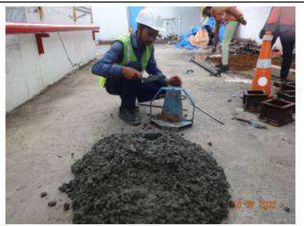
Figure 4&4: preparing concrete cube samples for testing and checking concrete slump
