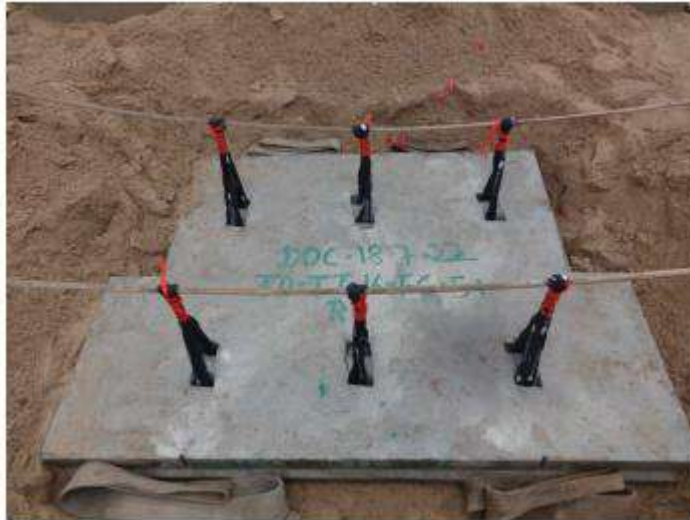
Figure 7: Panel Ready for testing, placed inside the test pit.
